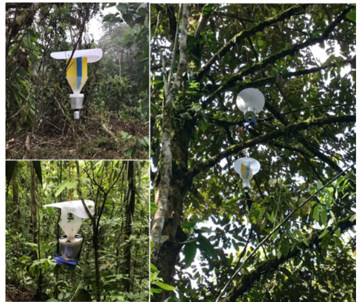
Figure 14: Insect traps installed in the Reassembly plots during the first fieldwork stage. Upper left: a mixed coloured bee vane trap, containing blue and yellow vanes; lower left: a mixed UV-light trap, which employs both UV and visible light to attract moths. Right: The traps installed in the canopy with the aid of a bow and arrow
